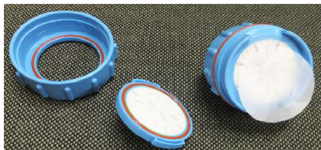
Figure4 : For air trapping Filter and holder
