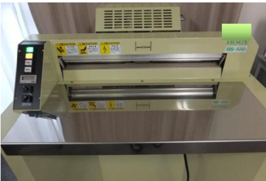
Figure2 : New conventional type sealer (Sealer for Gusset)
