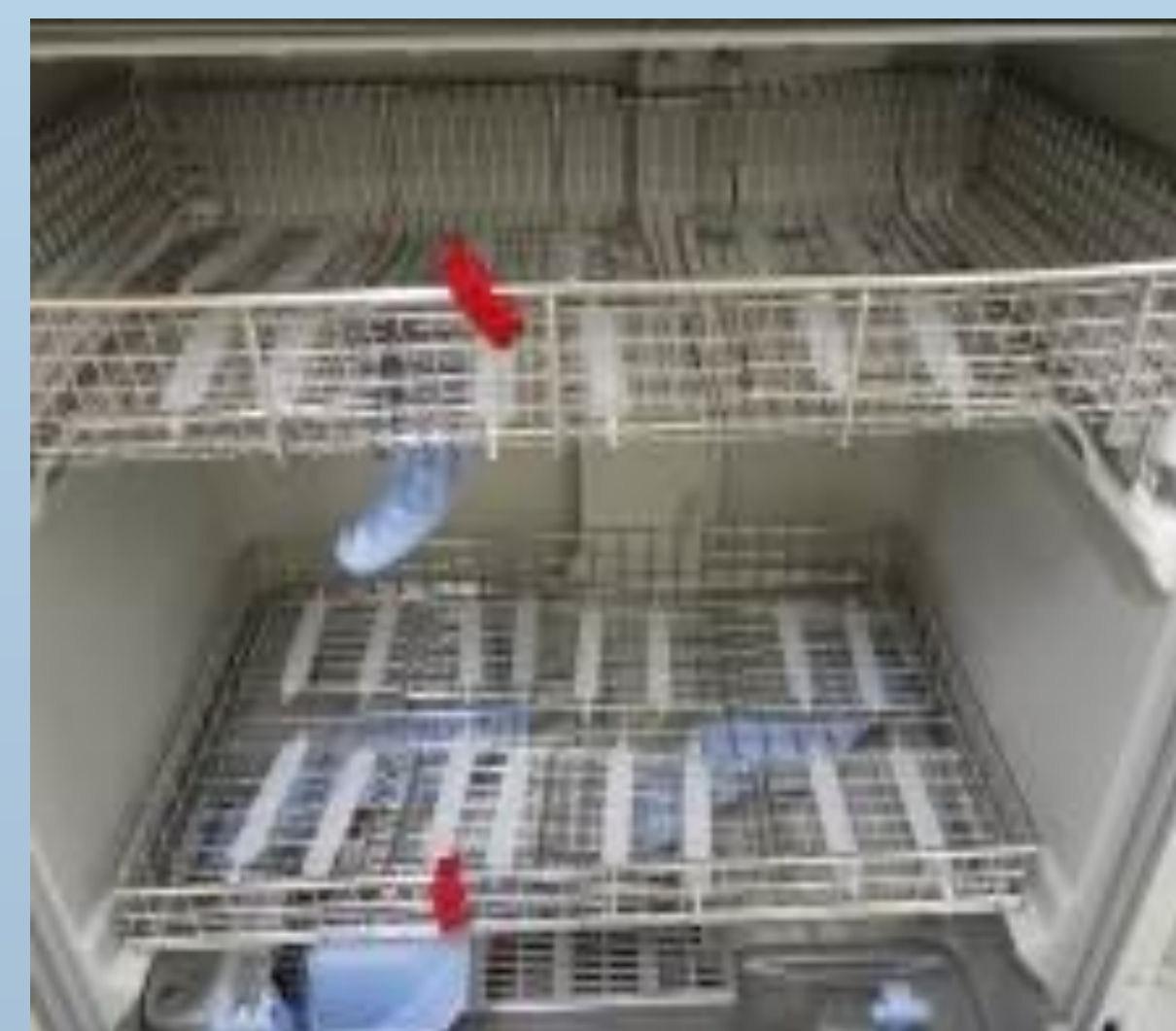
Figure 3. Layout Diagram of the Test Piece The test pieces smeared with the ATS of the upper and lower inside and were measured the residual hemoglobin after the washing.
