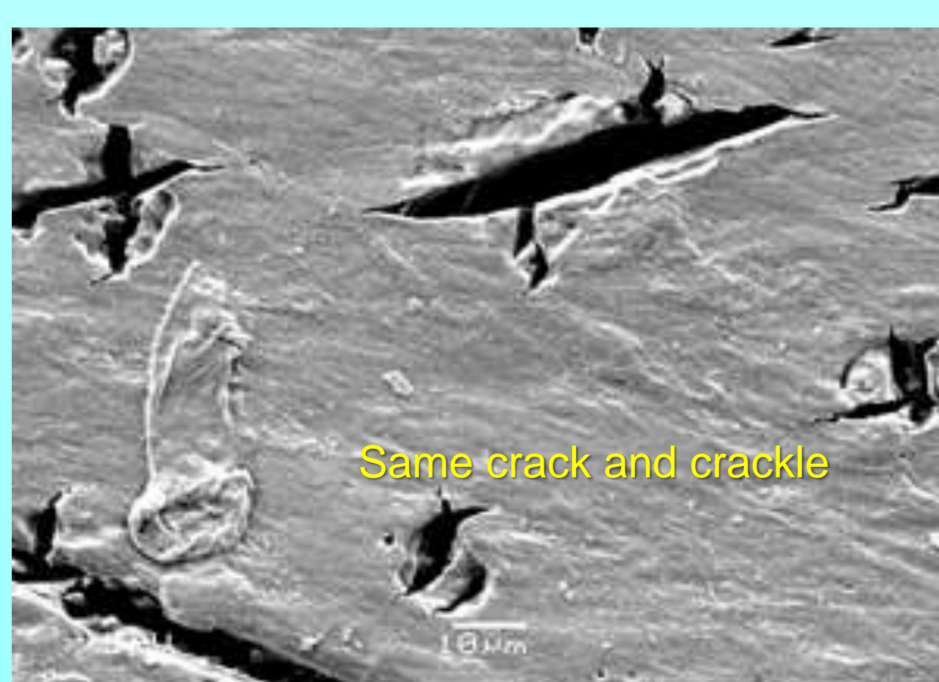
Figure1-4. SEMF of PA6 panel-surface after once of sterilisation by LTHPVS ( × 1000)
