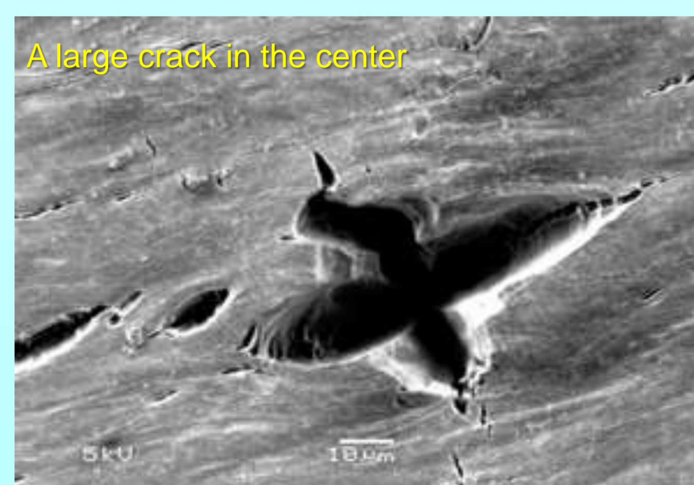
Figure 1-3. SEMF of PA6 panel-surface after five repeated procedures of sterilisation by LTHPGPS ( × 1000)
