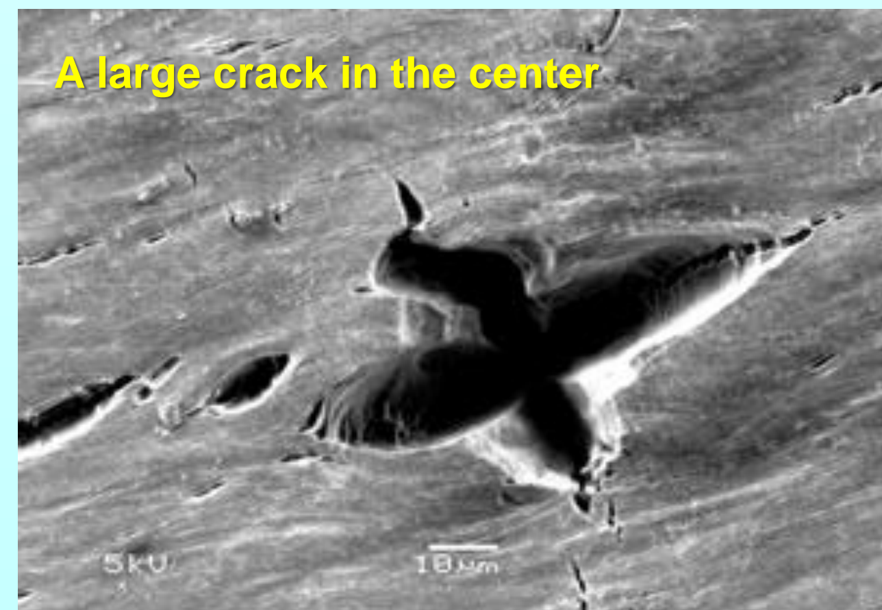
Figure 1-3. SEMF of PA6 panel-surface after five repeated procedures of sterilisation by LTHPGP (× 1000)
