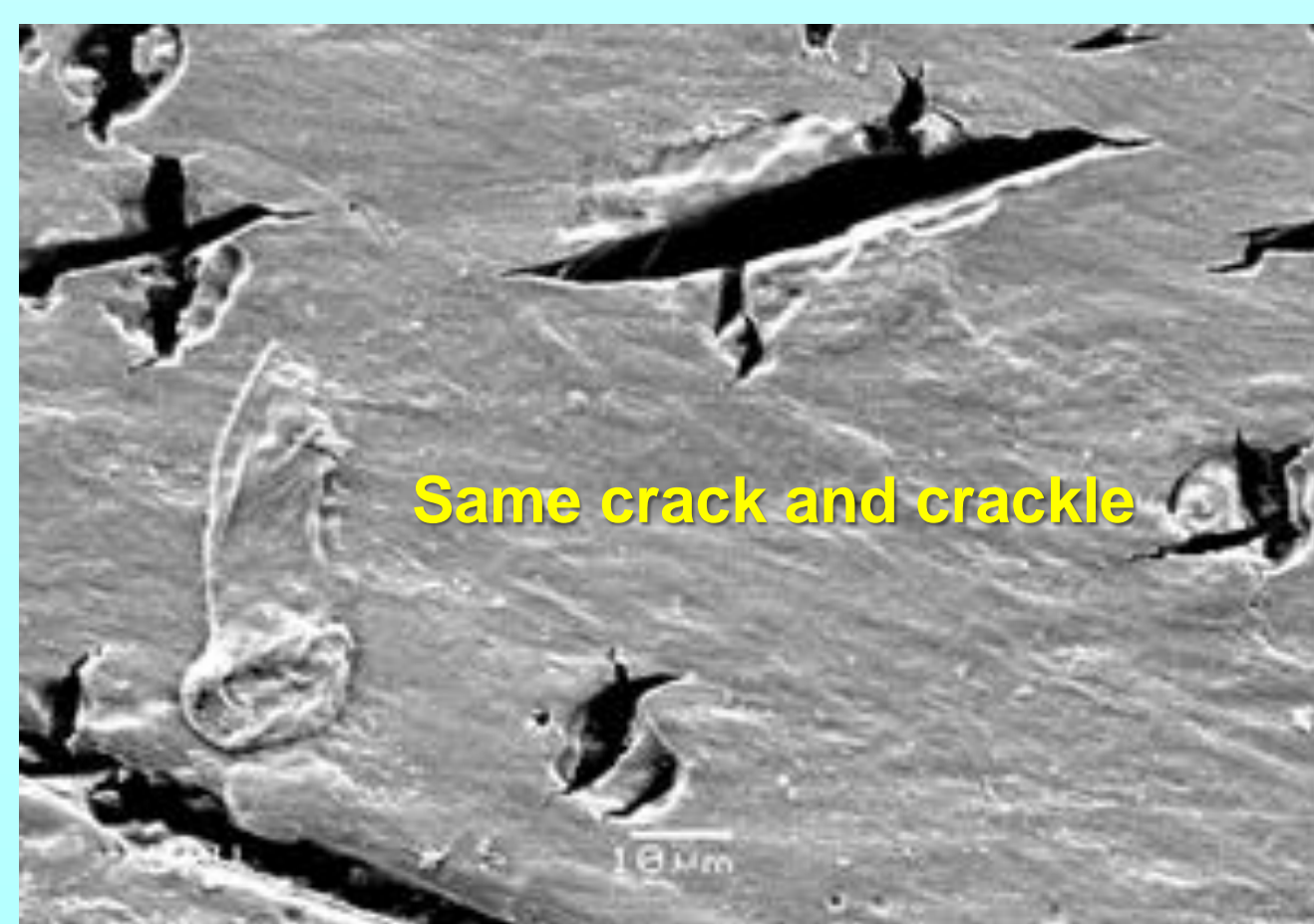
Figure 1-4. SEMF of PA6 panel-surface after once of sterilisation by LTHPV (× 1000)
