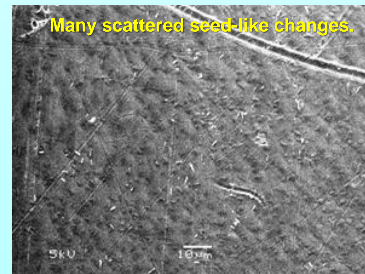
Figure 2-2. SEMF of PP panel-surface after five procedures of sterilisation by LTHPGP (× 1000)
